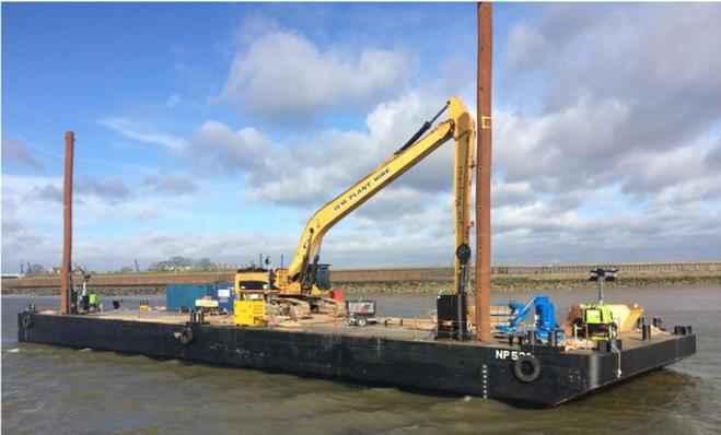
Neptune NP 531 Transfer barge with 2. No. 610.dia. hydraulically operated spud legs approx. depth 28.0m.
